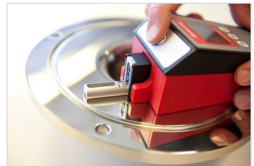
Illustration 4 – Measurement of the surface roughness
